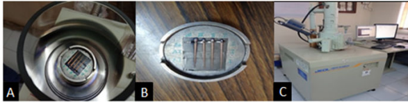
Figure 5: a) Gutta percha cones placed for gold coating; b) Gold coated gutta percha cones. c) Scanning Electron Microscope.
